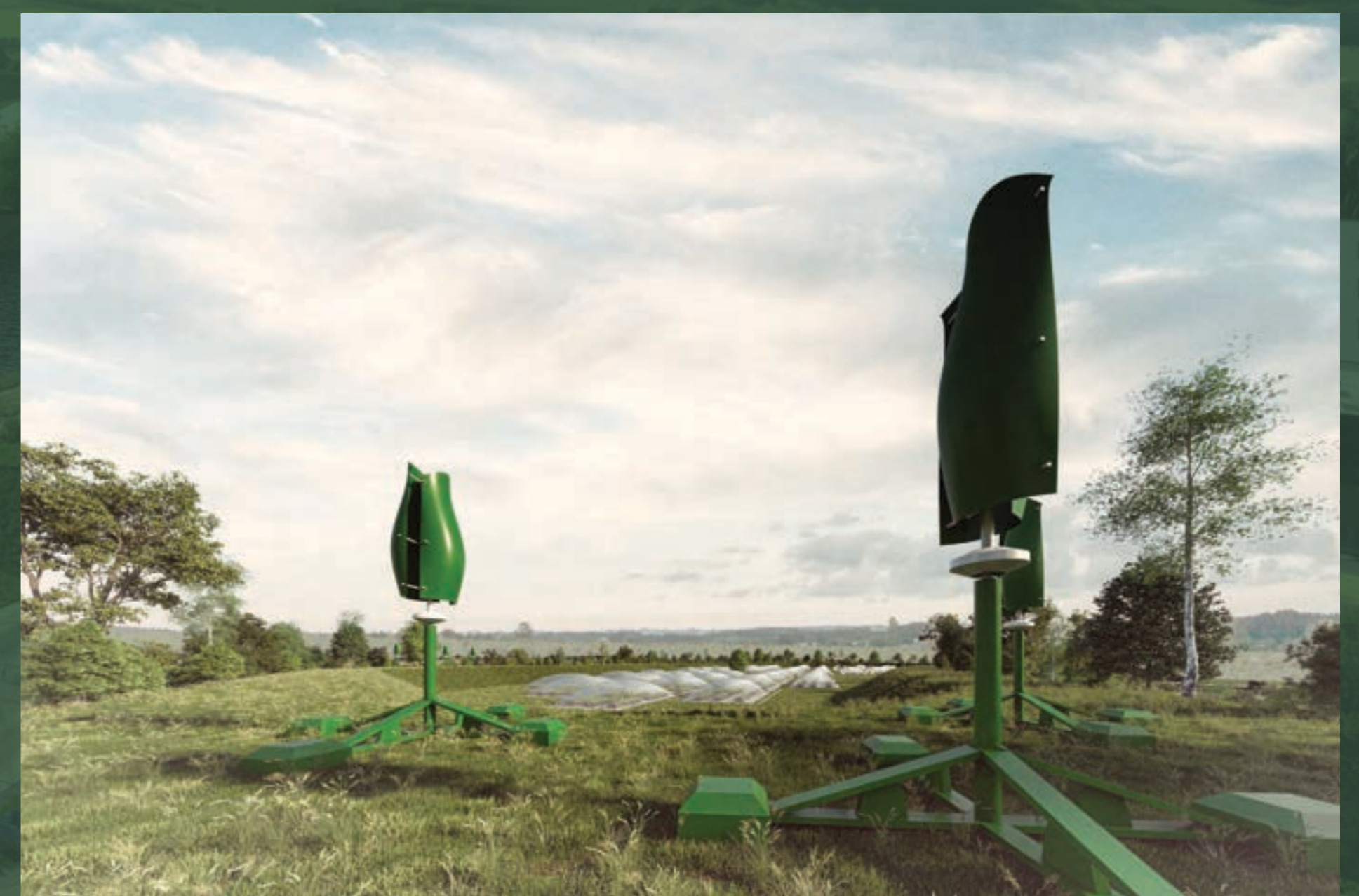
Innovative "Tulip" wind turbines can be installed with minimal foundations
